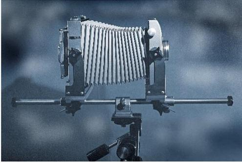
answer. You also could control perspective with this camera by moving the back standard. You also could control the plane of focus with the front standard. In 1975 I bought a 4x5" Calumet 22" bellows camera with a Caltar 215mm f/4.8 lens for product photography. I started learning how to use the view camera. This would put me ahead of many of the students in photography school by buying and learning how to use a view camera.
